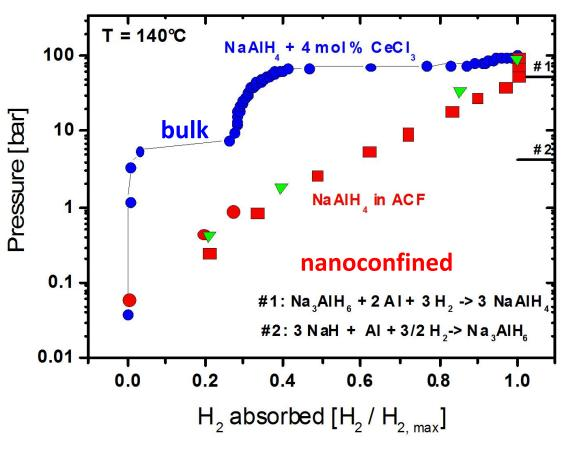
First experimental proof for modification of thermodynamics and reaction pathway of a nanoconfined complex hydride.
