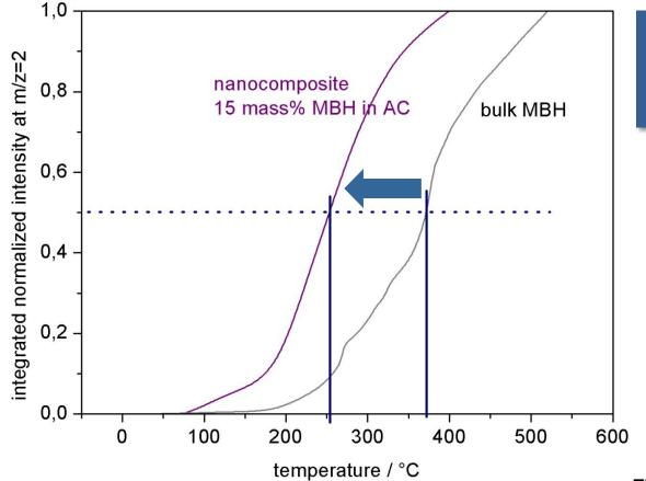
T shift of the H desorption by 120 K to lower temperatures !
