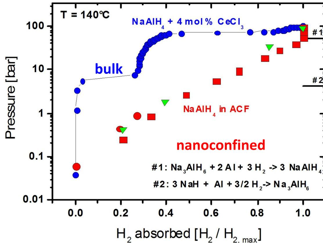
First experimental proof for modification of thermodynamics and reaction pathway of a nanoconfined complex hydride.
