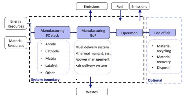
Figure 13: Boundary and processes for FC Systems
