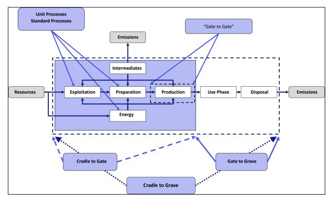
Figure 7: Possible system boundary in the life cycle of a product
