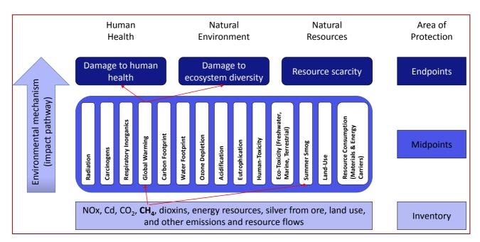
Figure 10: Schematic steps from Life Cycle Inventory to impact category (JRC 2010a) (modified)
