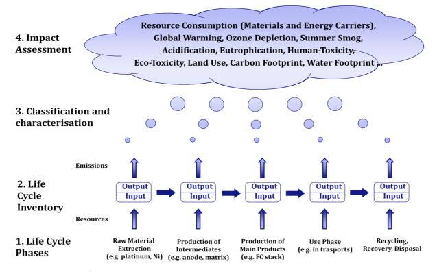
Figure 1: Overview of the LCA methodology
