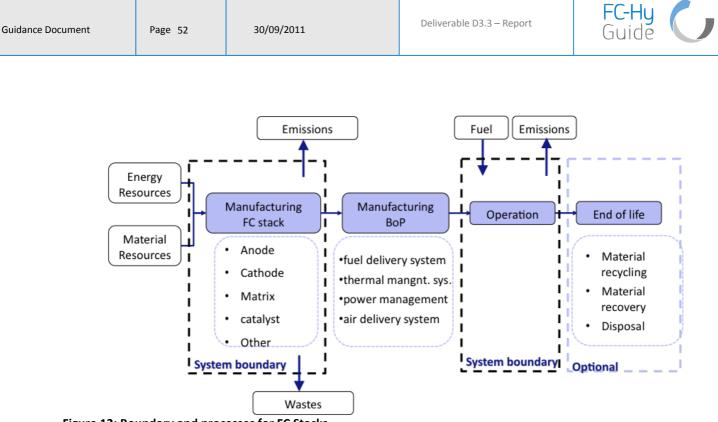
Figure 12: Boundary and processes for FC Stacks
