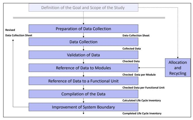
Figure 11: Simplified procedures for Lice Cycle Inventory Analysis (LCIA) (Source: ISO 2006b) (modified)
