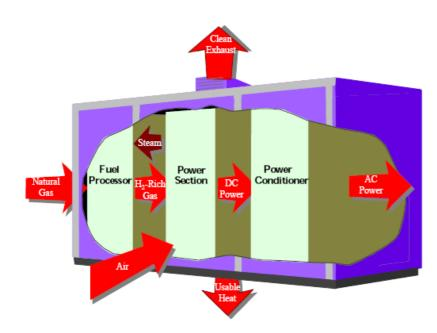
Figure 3: Schematic view of a generic fuel cell system (Source: Gasik 2008)
