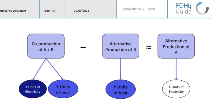
Figure 6: System expansion for solving multi-functionality (Source: JRC 2010) (modified)
