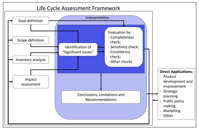
Figure 16: Relationship between elements within the interpretation phase and other phases of LCA (ISO 2006b) (modified)
