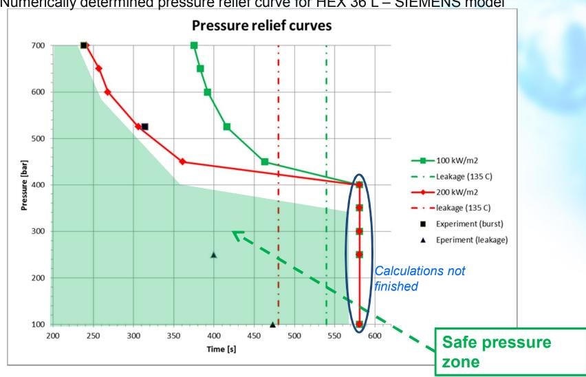
Numerically determined pressure relief curve for HEX 36 L – SIEMENS model
