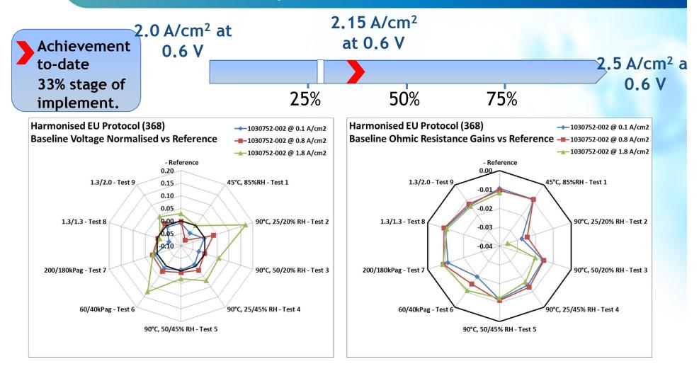
• MEA with baseline membrane using electrospun reinforcement and low EW Aquivion ionomer has demonstrated improved performance versus the project Reference MEA with conventional reinforcement, especially in hot dry conditions, and has also shown lower ohmic resistance.
