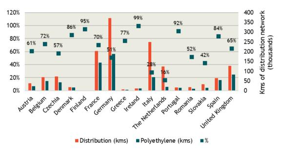
Figure 3-5 Share of polyethylene pipelines in distribution system. Source: Marcogaz technical statistics (2013)
