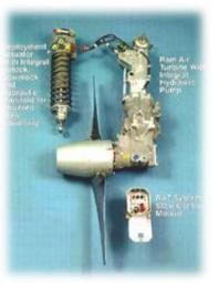
Ram Air Turbine (RAT) : wind turbine deployed in case of main electric supply failure, as an emergency system
