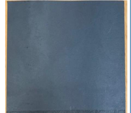
GDL non-uniformities not visible by optical approach but visible by thermography techniques
