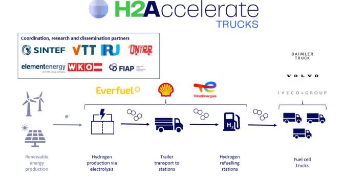
This project will fund the deployment of 150 fuel cell trucks across Europe by the mid-to-late 2020s, allowing development of the technology towards series manufacturing of the vehicles by the three major OEMs in the second half of the decade. The trucks to be deployed in the first stage are expected to be either 4x2 or 6x2, with up to 44 tonne capacity and long ranges of at least 600km.
