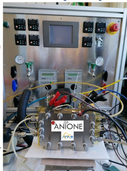
AEM ELECTROLYSIS single cell testing in ANIONE
