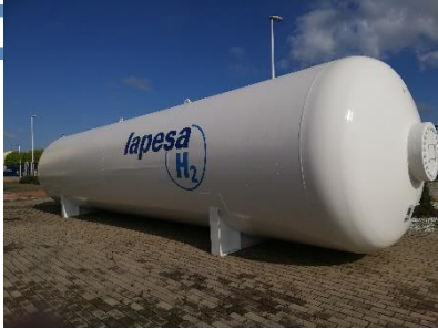
Buffer Tank 50 m 3 ; D:2450 L:11510 10-40 bar 180kg
