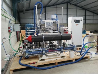
Compressor 50m 3 /h p_{in} : 10-40 bar p_{out} : 300-450 bar
