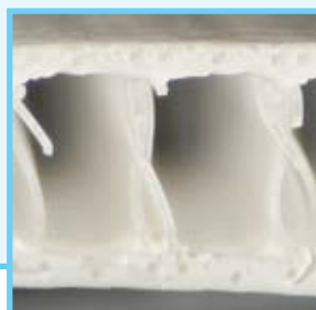
Cross section (left and middle) and top view of the E-bypass separator membrane for a 300 cm 2 electrolyser
