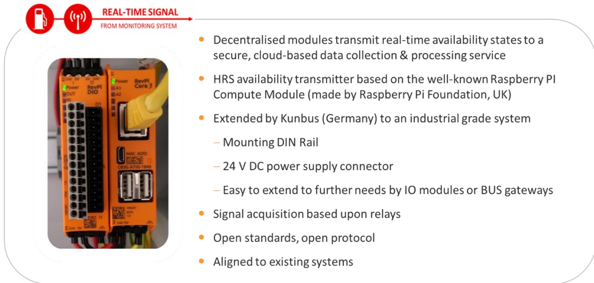
Figure 6: Overview of the RevPi hardware transmitter (type A HRS)
